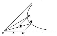
For the triangles CPL, CQM are equal, and, if PL meet CQ in R, it follows that the triangle CPR=the trapezium LRQM; hence, adding to each the area RPQ the theorem is proved.
